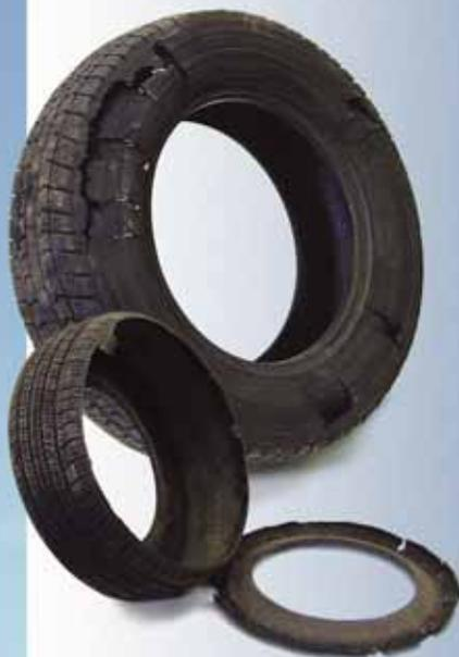
***Underinflation is the number one enemy of a tire. Operating an underinflated or overloaded tire at highway speeds on a warm summer day is a recipe for tire failure.***
