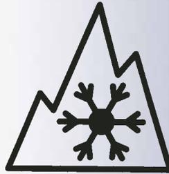
*Tires designed for use in snowy weather are marked with the peaked mountain with snowflake symbol.*
